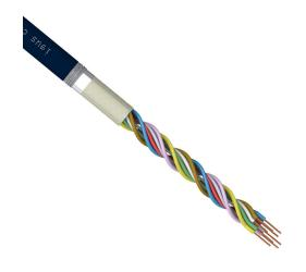
igus continuous flexing control and signal cable, shielded, 4 twisted pairs, 24 AWG (0.25mm2), 32-stranded, bare copper, TPE conductor insulation material, TPE jacket, blue, cut to length.
