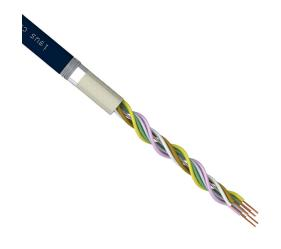
igus continuous flexing control and signal cable, shielded, 3 twisted pairs, 24 AWG (0.25mm2), bare copper, TPE conductor insulation material, pair 1: white and brown, pair 2: green and yellow and pair 3: grey and pink, TPE jacket, blue, cut to length.
