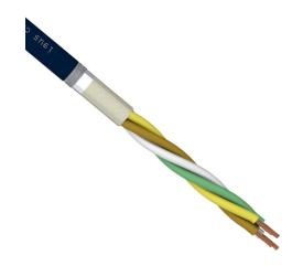
igus continuous flexing control and signal cable, shielded, 2 twisted pairs, 24 AWG (0.25mm2), bare copper, TPE conductor insulation material, pair 1: white and brown and pair 2: green and yellow, TPE jacket, blue, cut to length.
