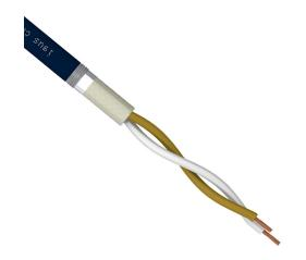
igus continuous flexing control and signal cable, shielded, 1 twisted pair, 24 AWG (0.25mm2), bare copper, TPE conductor insulation material, white and brown, TPE jacket, blue, cut to length.
