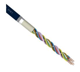
igus continuous flexing control and signal cable, shielded, 4 twisted pairs, 26 AWG (0.14mm2), 18-stranded, bare copper, TPE conductor insulation material, TPE jacket, blue, cut to length.
