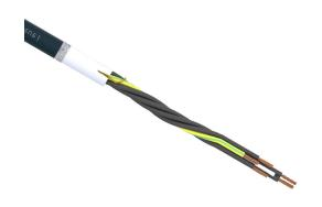
igus continuous flexing control cable, shielded, 5 conductors (includes ground), 16 AWG (1.50mm2), bare copper, TPE conductor insulation material, black with white numbers and green/yellow ground, TPE jacket, gray, cut to length.
