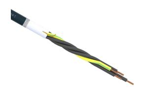
igus continuous flexing control cable, shielded, 4 conductors (includes ground), 16 AWG (1.50mm2), bare copper, TPE conductor insulation material, black with white numbers and green/yellow ground, TPE jacket, gray, cut to length.
