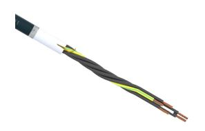
igus continuous flexing control cable, shielded, 5 conductors (includes ground), 18 AWG (0.75mm2), bare copper, TPE conductor insulation material, black with white numbers and green/yellow ground, TPE jacket, gray, cut to length.
