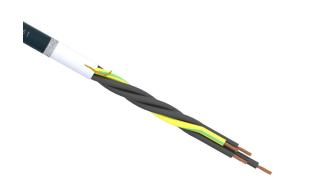
igus continuous flexing control cable, shielded, 4 conductors (includes ground), 18 AWG (0.75mm2), bare copper, TPE conductor insulation material, black with white numbers and green/yellow ground, TPE jacket, gray, cut to length.
