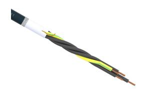
igus continuous flexing control cable, shielded, 4 conductors (includes ground), 18 AWG (0.75mm2), bare copper, TPE conductor insulation material, black with white numbers and green/yellow ground, TPE jacket, gray, cut to length.
