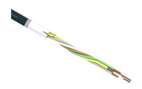
igus continuous flexing control cable, shielded, 5 conductors (includes ground), 20 AWG (0.50mm2), bare copper, TPE conductor insulation material, black with white numbers and green/yellow ground, TPE jacket, gray, cut to length.
