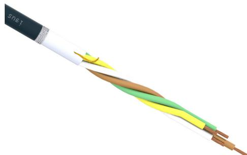
igus continuous flexing control cable, shielded, 4 conductors (includes ground), 20 AWG (0.50mm<sup>2</sup>), bare copper, TPE conductor insulation material, black with white numbers and green/yellow ground, TPE jacket, gray, cut to length.
