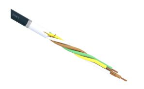
igus continuous flexing control cable, shielded, 4 conductors (includes ground), 20 AWG (0.50mm2), bare copper, TPE conductor insulation material, black with white numbers and green/yellow ground, TPE jacket, gray, cut to length.
