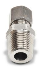
ProSense compression fitting, stainless steel, 1/2in male NPT process connection. For use with 10mm outside diameter temperature probes. Stainless steel ferrule included.
