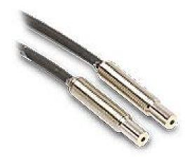
Micro Detectors optical fiber, plastic, cuttable, through-beam, M4 head, nickel-plated brass, polyethylene jacket, 120mm sensing distance, 2m length. Package of 2.
