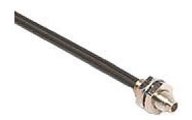
AutomationDirect optical fiber, plastic, cuttable, diffuse, M6 head, nickel-plated brass, polyethylene jacket, 260mm sensing distance, 2m length.
