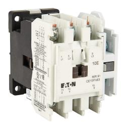
Eaton Freedom series IEC contactor, 32A, (3) N.O. power poles, (1) N.O. auxiliary contacts, 240 VAC (60Hz)/220 VAC (50Hz) coil voltage.
