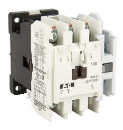
Eaton Freedom series IEC contactor, 32A, (3) N.O. power poles, (1) N.O. auxiliary contacts, 120 VAC (60Hz)/110 VAC (50Hz) coil voltage.
