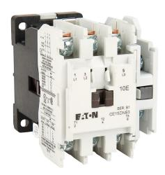
Eaton Freedom series IEC contactor, 18A, (3) N.O. power poles, (1) N.O. auxiliary contacts, 120 VAC (60Hz)/110 VAC (50Hz) coil voltage.
