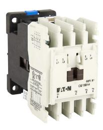
Eaton Freedom series IEC contactor, 10A, (4) N.O. power poles, 240 VAC (60Hz)/220 VAC (50Hz) coil voltage.
