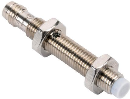
ProSense capacitive proximity sensor, tubular, 8mm diameter x 54mm body, stainless steel housing, PNP, N.C. output, 3mm sensing distance, non-flush, 100 Hz switching frequency, IP65, 3-pin M8 quick-disconnect.
