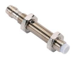
ProSense capacitive proximity sensor, tubular, 8mm diameter x 54mm body, stainless steel housing, PNP, N.C. output, 3mm sensing distance, non-flush, 100 Hz switching frequency, IP65, 3-pin M8 quick-disconnect.
