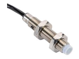
ProSense capacitive proximity sensor, tubular, 8mm diameter x 42mm body, stainless steel housing, PNP, N.C. output, 3mm sensing distance, non-flush, 100 Hz switching frequency, IP65, pigtail.
