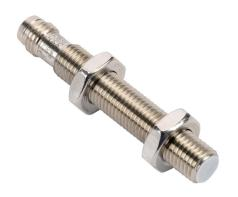
ProSense capacitive proximity sensor, tubular, 8mm diameter x 54mm body, stainless steel housing, PNP, N.C. output, 1.5mm sensing distance, flush, 100 Hz switching frequency, IP65, 3-pin M8 quick-disconnect.
