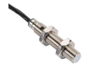
ProSense capacitive proximity sensor, tubular, 8mm diameter x 42mm body, stainless steel housing, PNP, N.C. output, 1.5mm sensing distance, flush, 100 Hz switching frequency, IP65, pigtail.
