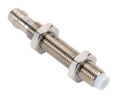
ProSense capacitive proximity sensor, tubular, 8mm diameter x 54mm body, stainless steel housing, PNP, N.O. output, 3mm sensing distance, non-flush, 100 Hz switching frequency, IP65, 3-pin M8 quick-disconnect.
