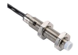
ProSense capacitive proximity sensor, tubular, 8mm diameter x 42mm body, stainless steel housing, PNP, N.O. output, 3mm sensing distance, non-flush, 100 Hz switching frequency, IP65, pigtail.
