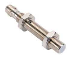
ProSense capacitive proximity sensor, tubular, 8mm diameter x 54mm body, stainless steel housing, PNP, N.O. output, 1.5mm sensing distance, flush, 100 Hz switching frequency, IP65, 3-pin M8 quick-disconnect.
