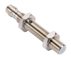
ProSense capacitive proximity sensor, tubular, 8mm diameter x 54mm body, stainless steel housing, PNP, N.O. output, 1.5mm sensing distance, flush, 100 Hz switching frequency, IP65, 3-pin M8 quick-disconnect.
