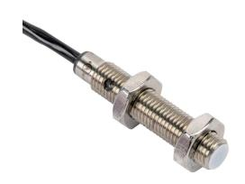
ProSense capacitive proximity sensor, tubular, 8mm diameter x 42mm body, stainless steel housing, PNP, N.O. output, 1.5mm sensing distance, flush, 100 Hz switching frequency, IP65, pigtail.
