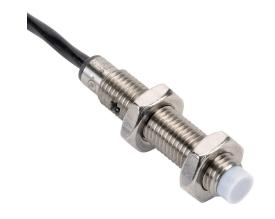
ProSense capacitive proximity sensor, tubular, 8mm diameter x 42mm body, stainless steel housing, NPN, N.O. output, 3mm sensing distance, non-flush, 100 Hz switching frequency, IP65, pigtail.
