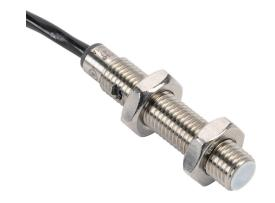
ProSense capacitive proximity sensor, tubular, 8mm diameter x 42mm body, stainless steel housing, NPN, N.O. output, 1.5mm sensing distance, flush, 100 Hz switching frequency, IP65, pigtail.
