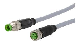
AutomationDirect connection cable, M8 axial female to axial male, 3-pole, PVC jacket, gray, 3.2ft/1m cable length, IP67.
