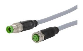
AutomationDirect connection cable, M8 axial female to axial male, 3-pole, PVC jacket, gray, 3.2ft/1m cable length, IP67.
