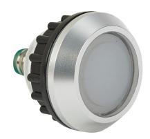
Captron LED indicating light, permanent light function, IP69K, 22mm, red/green, 28mm, round, plastic base, aluminum bezel, 24 VDC, full voltage. Requires M8 4-pole connection cable.
