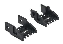
Murrplastik bracket, 1.02in inside height, 1.46in inside width, polyamide, black. For use with MP3000 series energy chain.
