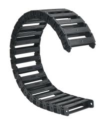
Murrplastik MP3000 cable drag chain, 1.02in inside height, 4.92in inside width, 7.9in bend radius, inside opening, 1.77in pitch, 3.2ft/1m length, black. Requires CDC-KAZ-10X49 bracket for mounting.
