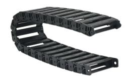
Murrplastik MP3000 cable drag chain, 1.02in inside height, 4.92in inside width, 2.8in bend radius, inside opening, 1.77in pitch, 3.2ft/1m length, black. Requires CDC-KAZ-10X49 bracket for mounting.
