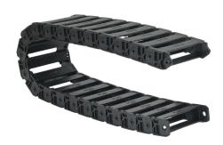
Murrplastik MP3000 cable drag chain, 1.02in inside height, 3.98in inside width, 2.8in bend radius, inside opening, 1.77in pitch, 3.2ft/1m length, black. Requires CDC-KAZ-10X40 bracket for mounting.
