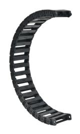
Murrplastik MP3000 cable drag chain, 1.02in inside height, 3.98in inside width, 11.8in bend radius, inside opening, 1.77in pitch, 3.2ft/1m length, black. Requires CDC-KAZ-10X40 bracket for mounting.
