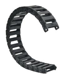
Murrplastik MP3000 cable drag chain, 1.02in inside height, 3.43in inside width, 7.9in bend radius, inside opening, 1.77in pitch, 3.2ft/1m length, black. Requires CDC-KAZ-10X34 bracket for mounting.
