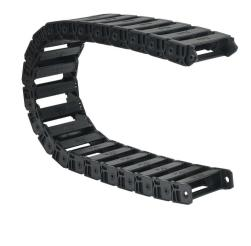
Murrplastik MP3000 cable drag chain, 1.02in inside height, 3.43in inside width, 4.7in bend radius, inside opening, 1.77in pitch, 3.2ft/1m length, black. Requires CDC-KAZ-10X34 bracket for mounting.
