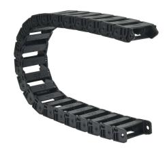
Murrplastik MP3000 cable drag chain, 1.02in inside height, 3in inside width, 4.7in bend radius, inside opening, 1.77in pitch, 3.2ft/1m length, black. Requires CDC-KAZ-10X30 bracket for mounting.
