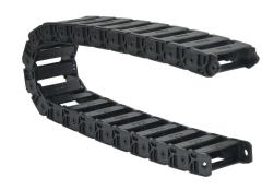
Murrplastik MP3000 cable drag chain, 1.02in inside height, 3in inside width, 2.8in bend radius, inside opening, 1.77in pitch, 3.2ft/1m length, black. Requires CDC-KAZ-10X30 bracket for mounting.
