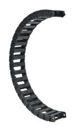
Murrplastik MP3000 cable drag chain, 1.02in inside height, 3in inside width, 11.8in bend radius, inside opening, 1.77in pitch, 3.2ft/1m length, black. Requires CDC-KAZ-10X30 bracket for mounting.
