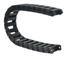
Murrplastik MP3000 cable drag chain, 1.02in inside height, 2.44in inside width, 4.7in bend radius, inside opening, 1.77in pitch, 3.2ft/1m length, black. Requires CDC-KAZ-10X24 bracket for mounting.
