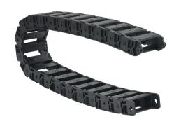
Murrplastik MP3000 cable drag chain, 1.02in inside height, 2.44in inside width, 2.8in bend radius, inside opening, 1.77in pitch, 3.2ft/1m length, black. Requires CDC-KAZ-10X24 bracket for mounting.
