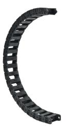
Murrplastik MP3000 cable drag chain, 1.02in inside height, 2.44in inside width, 11.8in bend radius, inside opening, 1.77in pitch, 3.2ft/1m length, black. Requires CDC-KAZ-10X24 bracket for mounting.
