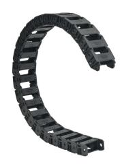
Murrplastik MP3000 cable drag chain, 1.02in inside height, 2.2in inside width, 7.9in bend radius, inside opening, 1.77in pitch, 3.2ft/1m length, black. Requires CDC-KAZ-10X22 bracket for mounting.
