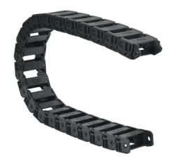
Murrplastik MP3000 cable drag chain, 1.02in inside height, 2.2in inside width, 4.7in bend radius, inside opening, 1.77in pitch, 3.2ft/1m length, black. Requires CDC-KAZ-10X22 bracket for mounting.
