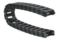
Murrplastik MP3000 cable drag chain, 1.02in inside height, 2.2in inside width, 2.8in bend radius, inside opening, 1.77in pitch, 3.2ft/1m length, black. Requires CDC-KAZ-10X22 bracket for mounting.
