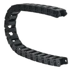
Murrplastik MP3000 cable drag chain, 1.02in inside height, 1.46in inside width, 4.7in bend radius, inside opening, 1.77in pitch, 3.2ft/1m length, black. Requires CDC-KAZ-10X15 bracket for mounting.
