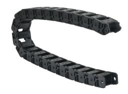
Murrplastik MP3000 cable drag chain, 1.02in inside height, 1.46in inside width, 2.8in bend radius, inside opening, 1.77in pitch, 3.2ft/1m length, black. Requires CDC-KAZ-10X15 bracket for mounting.
