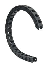
Murrplastik MP3000 cable drag chain, 1.02in inside height, 1.02in inside width, 7.9in bend radius, inside opening, 1.77in pitch, 3.2ft/1m length, black. Requires CDC-KAZ-10X10 bracket for mounting.
