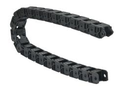
Murrplastik MP3000 cable drag chain, 1.02in inside height, 1.02in inside width, 2.8in bend radius, inside opening, 1.77in pitch, 3.2ft/1m length, black. Requires CDC-KAZ-10X10 bracket for mounting.
